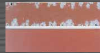
(TOP) SINGLE-COAT POLYESTER OVER METAL FROM A SCRAP-BASED MINI-MILL (BOTTOM) ALUMALURE 2000 PANEL
